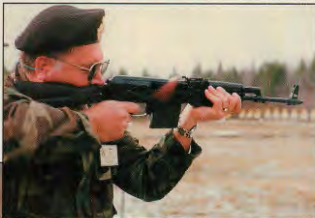
(right) A .410-gauge semiautomatic shotgun of the SAIGA family. Based upon the Kalashnikov method of operation and sharing some parts interchangeability with the AK, this particular version has been configured as an AK and is already in service with border-guard units of several states of the CIS. (below) Victor Kalashnikov, son of Mikhail T. Kalashnikov who, together with Alexi Dragunov, youngest son of Evgeni F. Dragunov, designed the Bizon submachine gun with its unique helical-type magazine, shown here with a sound-suppressed version of his design.
